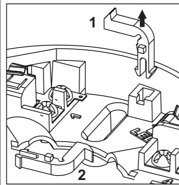
The mounting base includes an optional feature to prevent the removal of the detector without the use of a tool.
