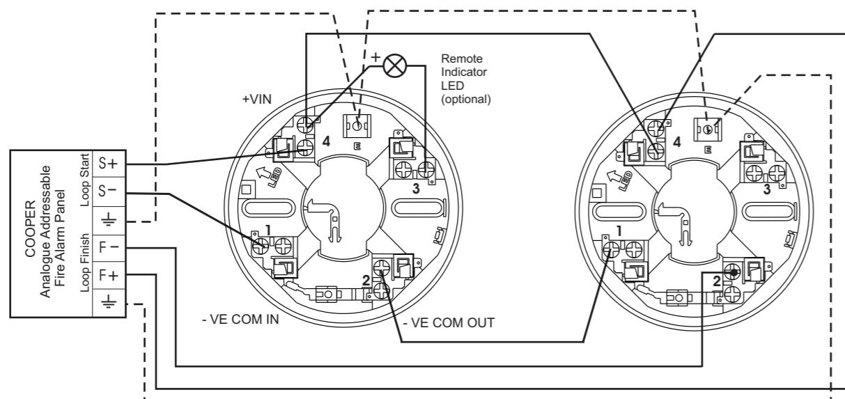
Attention: If using the outer connection on terminal 2, ensure the operation of the switch is not impeded and that there no shorts between terminal 2 and the switch contact.
